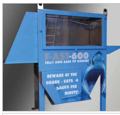
MATERIALS OF CONSTRUCTION - GENERALLY SS304/ACETAL COPOLYMER OVERALL EXTERNAL FINISH - SS304 180 GRIT OR  $0.8\mu m$  / INTERNAL FINISH TO  $0.4\mu m$ /MILL FINISH 240 GRIT OR 2B/DAIRY
