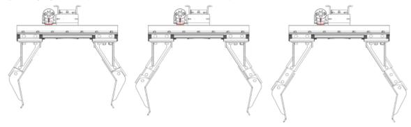
The Clamping Ranges for each Arm, in each of the 3 Pin Positions is shown in the table: The shortest Arm, gives positions 1-3, the middle Arm gives positions 2-4 and the longest, positions 3-5.
