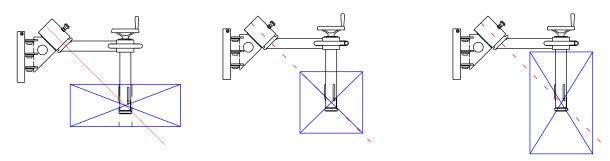
As a roll becomes wider, it must use a longer Box Arm to stay in balance. Torros offers 2 standard lengths of Box Arm, 350mm and 435mm which cover most roll sizes.
