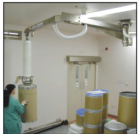
Fibre keg, plastic drum and sack handling vacuum lifter supported from a ceiling mounted 360° rotational articulated arm, manufactured in 304 stainless steel.
