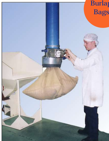
Vacuum Lifter - with spike gripper feature
