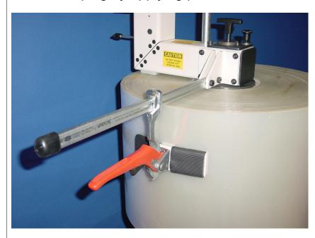
To operate, simply slide the clamp into place against the roll O.D. and lift the handle. The handle ratchets firmly in place. To release the clamp, simply pull the trigger.
