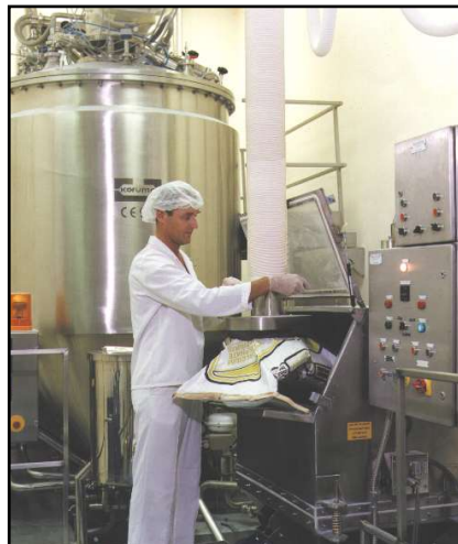
Wall mounted swing jib arrangement and vacuum tube lifter handling sacks from a pallet into a sack tip booth.
