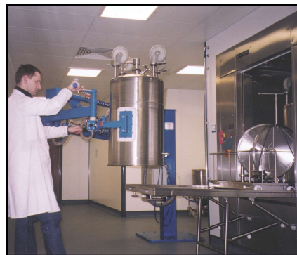
Low level manipulator lifting and inverting stainless steel vessels and feeding into washing machine.
