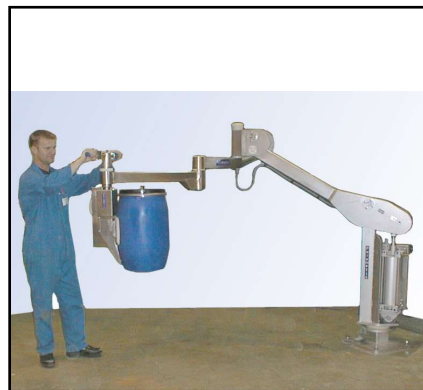
Stainless Steel Manipulator with weighing feature handling plastic drums from a filling head to a pallet.
