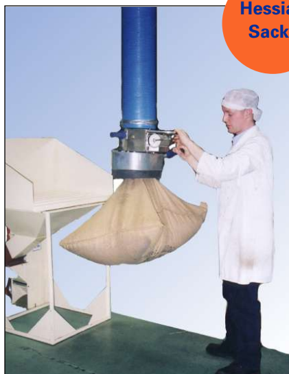
Vacuum Lifter - with spike gripper feature
