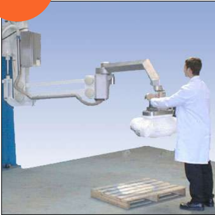
Manipulator - suitable for low headroom situations
