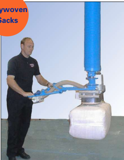
Vacuum Lifter - with extended handle feature for high stacking
