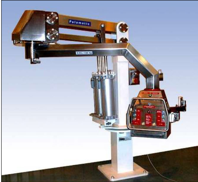
Manipulator designed to pour a range of drum sizes and to lift paper and plastic sacks. The unit gripped product pneumatically and by vacuum. Also incorporated HEPA filtration. The system was installed for use in a containment booth environment.
