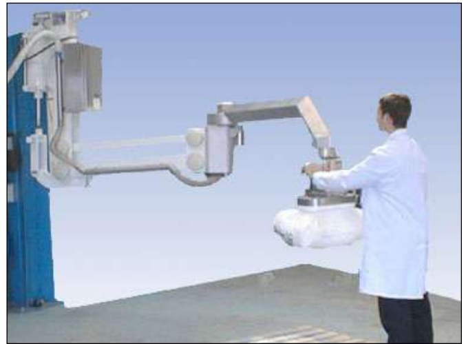
Inverted manipulator suitable for suspending from overhead steelwork. The system incorporated vacuum grip to easily handle a range of drums and sacks. This unit had a SWL of up to 210kg.
