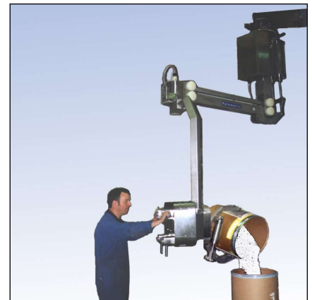
Inverted manipulator suitable for suspending from overhead steelwork. The system incorporated vacuum grip to easily handle a range of drums and sacks. This unit had a SWL of up to 210kg.
