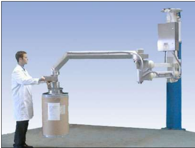
Inverted manipulator suitable for suspending from overhead steelwork. The system incorporated vacuum grip to easily handle a range of drums and sacks. This unit had a SWL of up to 210kg.
