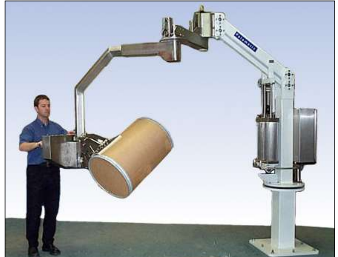
This unit was designed to lift and pour the contents of a range of fibre kegs weighing up to 70kg directly into a reactor. The system requires compressed air for operation making it suitable for flameproof and zone 21 environments.
