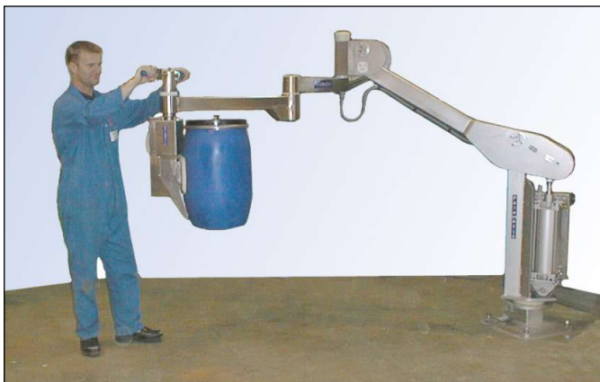
Inverted manipulator suitable for suspending from overhead steelwork. The system incorporated vacuum grip to easily handle a range of drums and sacks. This unit had a SWL of up to 210kg.
