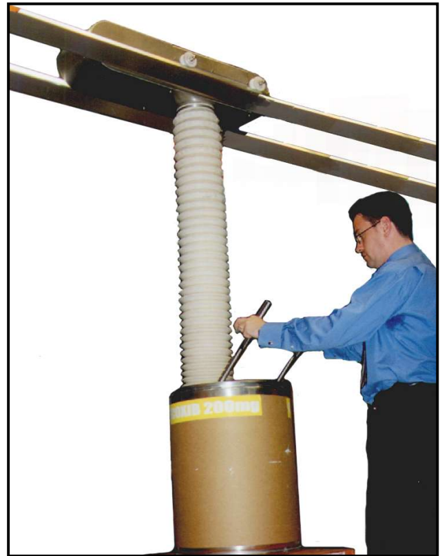
Example of Palamatic's PneuHoist-C (Compact version). Pneumatically actuated gripping jaws are used to securely grip the plastic bag before it is lifted clear of the keg and placed on an adjacent dispensing table.
