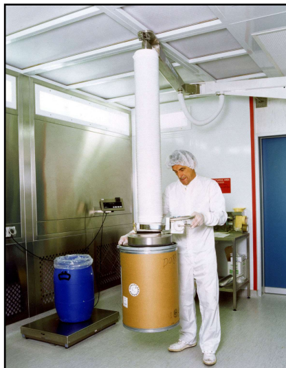
Palamatic Vacuum Tube Lifter. Effortless and safe handling of fibre kegs within a dispensary booth
