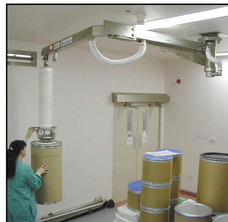
Fibre keg, plastic drum and sack handling vacuum lifter supported from a ceiling mounted 360° rotational articulated arm, manufactured in 304 stainless steel.
