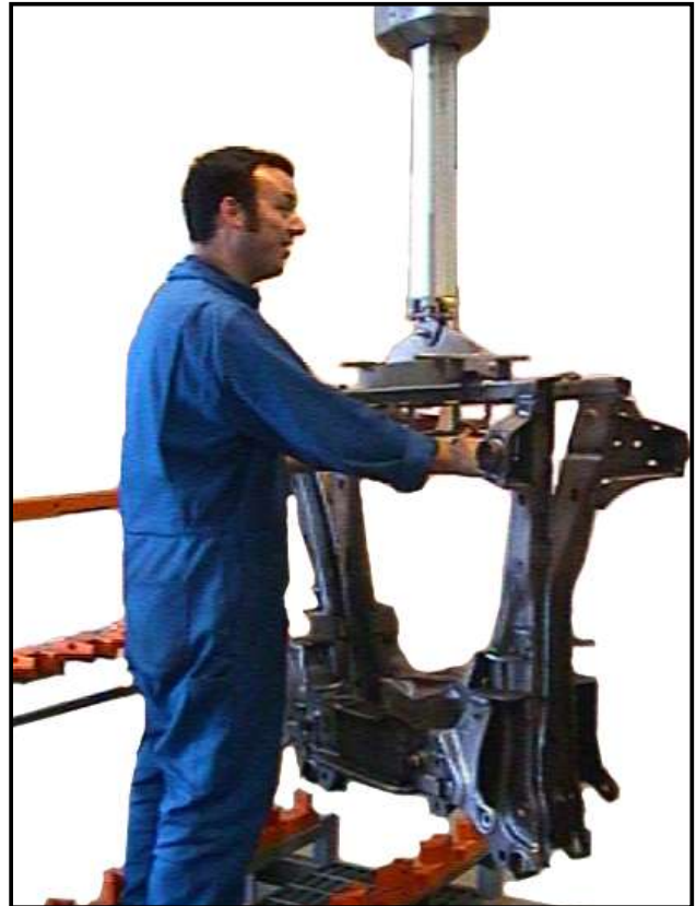
Operator controls are conveniently positioned to ensure ease of use. Raising and lowering of the sub frame is achieved via push-button controls, as is the pneumatic gripping mechanism used to secure the load during the transfer process.
