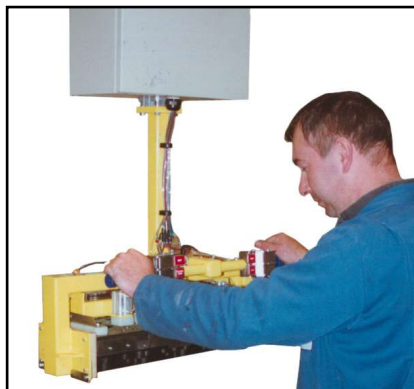
PneuLift used to handle 35kg cylinder heads with precise and horizontal positioning onto the cylinder block
