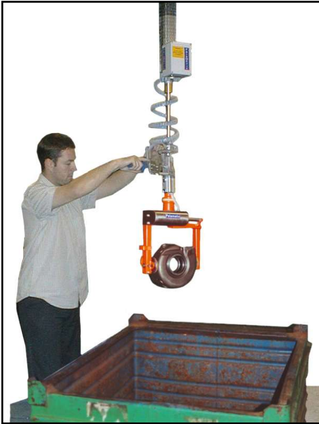
Palamatic's PneuLift transferring Turbo Casings from stillage to stillage. In this operation the Turbo Casings, weighing 40kgs, will be rotated through 180° during the transfer process. When installed the unit will be suspended from an overhead gantry providing maximum working area coverage with the minimum disruption to the operating environment.
