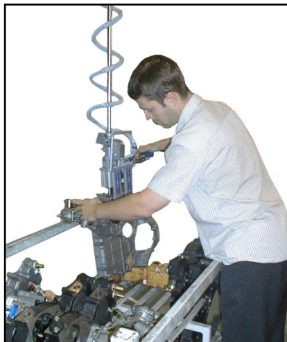
Typical application picking from stillage to engine block with components picked in a vertical orientation
