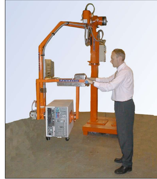
Computer server manipulated before final assembly. Both pneumatic and vacuum grip to ensure safe handling.
