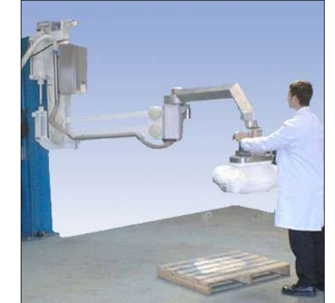
Inverted manipulator suitable for suspending from overhead steelwork. The system incorporated vacuum grip to easily handle a range of drums and sacks. This unit had a SWL of up to 210kg.
