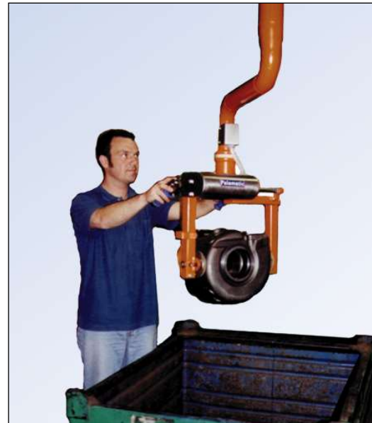
90° reel Manipulator loading mandrel. Unit features special 'pushing' mechanism to positively feed reel onto machine mandrel
