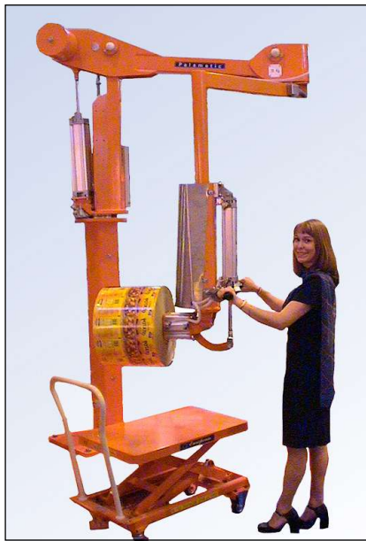
Manipulator complete with reel core gripper and 90° rotation
