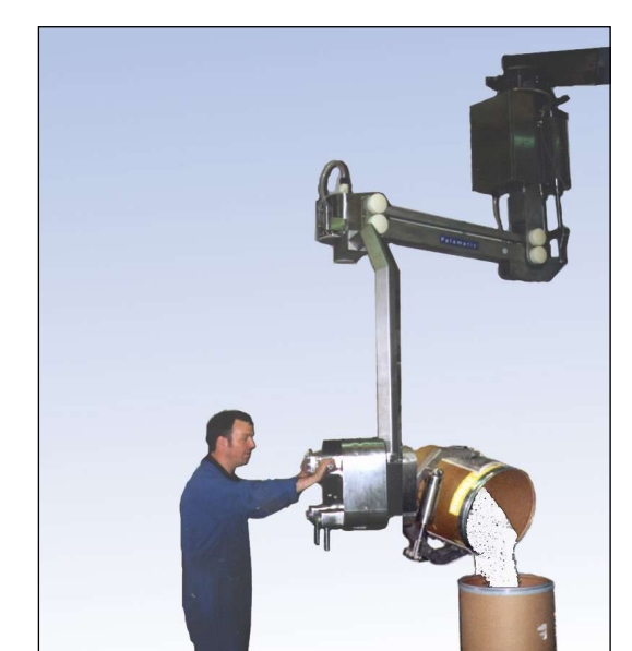
This unit was designed to lift and pour the contents of a range of fibre kegs weighing up to 70kg directly into a reactor. The system requires compressed air for operation making it suitable for flameproof and zone 21 environments.
