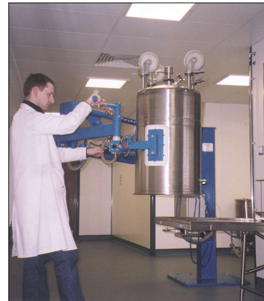
180° Manual rotation allowing operator to load and unload stainless steel bins in and out of washing process in a clean room environment.
