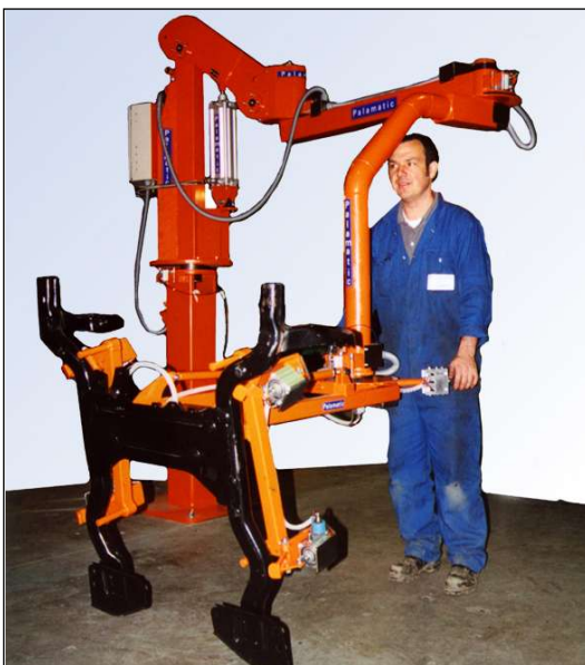
HRA type Manipulator lifting and turning sub frame assemblies for the Automotive industry.
