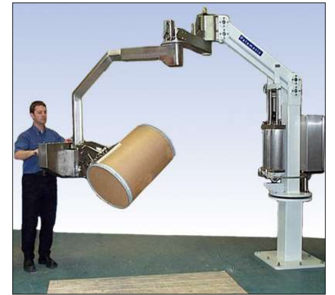
This unit was designed to lift and pour the contents of a range of fibre kegs weighing up to 70kg directly into a reactor. The system requires compressed air for operation making it suitable for flameproof and zone 21 environments.
