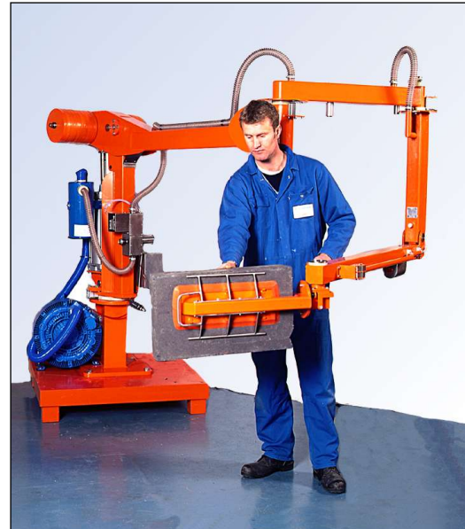
Manipulator handling refractory bricks. Features additional reach cantilever with manual rotation built in to end effector. System is also mobile, via fork or
