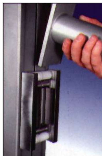
Quick release mechanism for rapid arm changeover
