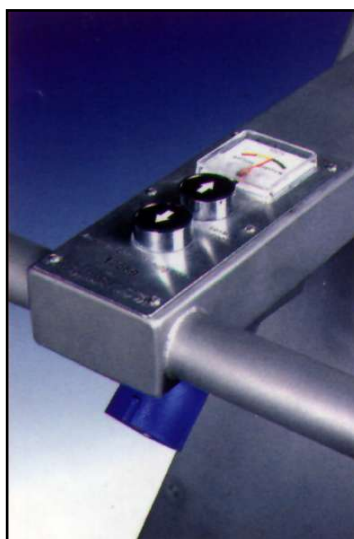
Push button controls, battery level indicator and charging point
