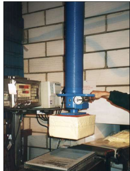
Example - Vacuum Tube Lifters; this system installed in the Fisheries sector enables operator to stack 45kg boxed salmon up to six layers high on pallets.
