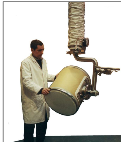
Side vacuum grip of the keg allows the operator to manually tip the product from the keg into a discharge station.
