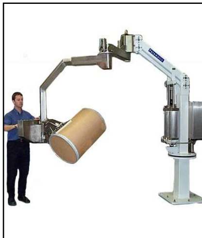
Manipulator used to lift and pour various drums and kegs in to a filter dryer in a GMP process area. Operator has complete control over the pouring function in a safe and weightless lifting process.
