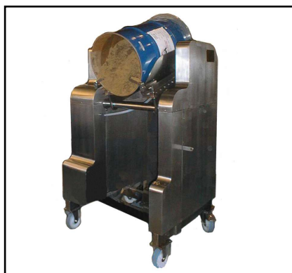
Mobile DrumTipper handling 45G steel drum. Drum is loaded onto a cradle and secured before inversion takes place. This pneumatically powered unit also features a 'drum shake' facility to ensure positive discharge of product.
