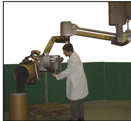
Stainless Steel Manipulator used to lift and pour fibre kegs. Operator has complete control over the pouring function in a safe and weightless lifting process.
