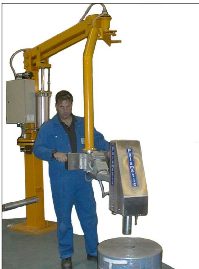
Palamatic provided a solution at the Black Sheep Brewery for handling full casks. Horizontal casks are turned upright and then palletised.
