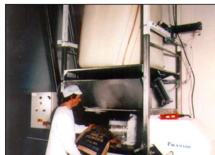
Automatic sack discharging machines which are suitable for handling filter aid such as diatomaceous earth in a dust tight process. An operator exposure level report identified the requirement for contained handling of this carcinogenic product within brewing and wine making industries.
