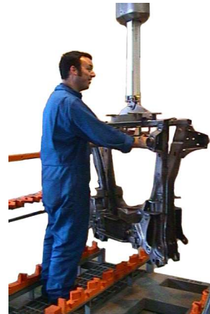
REF NO: PL-PG-010 FEATURES: PneuLift lifting sub frames from conveyor and placing in stillage
