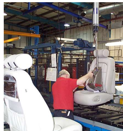
REF NO: PL-PG-006 FEATURES: PneuLift handling 28kg car seats from conveyor to packing area mounted on 25 x 3m 'H' style gantry
