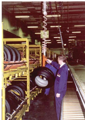
REF NO: PL-MG-011 FEATURES: PneuLift lifting green tyres from conveyor to racking
