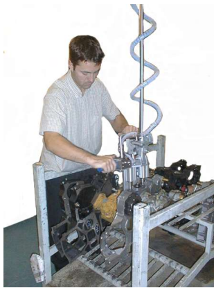
REF NO: PL-PG-007 FEATURES: PneuLift with pneumatic grip handling 30kg automotive components from stillage to engine block
