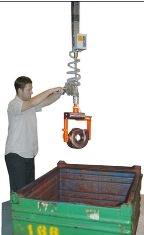
REF NO: PL-PG-003 FEATURES: PneuLift lifting turbo castings from stillage to milling machine
