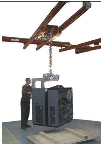
REF NO: CPL-MG-001 FEATURES: Compact PneuLift handling 400kg liquid coolers from production line to a pallet. Supported from a double girder bridge beam
