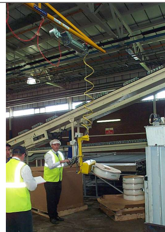
REF NO: CPL-VG-006 FEATURES: Compact PneuLift handling Hi-Cone reels from horizontal to vertical o load packaging machine
