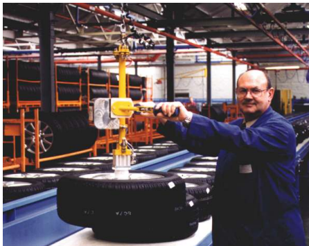
REF NO: CPL-PG-003 FEATURES: 63 and 75mm pneumatic tyre gripper suspended from Compact PneuLift on a 38m x 4m 'H' Style gantry system
