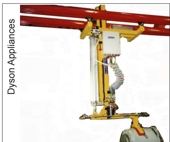
REF NO: PIL-VG-006 FEATURES: Pillar Lift handling washing machine drum from conveyor and placing in main support frame. 70kg SWL
