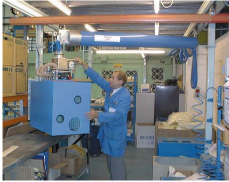
REF NO: HT-VG-001 FEATURES: Horizontal vacuum tube lifter mounted on H style gantry under mezzanine floor
