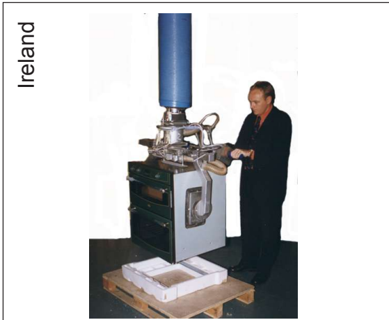
REF NO: E-CG-002 WEIGHT: 20kg FEATURES: Pneumatic and vacuum grip handling ovens on either side
