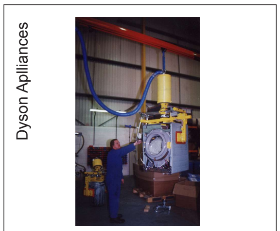
REF NO: E-CG-005 WEIGHT: 20kg FEATURES: Vacuum and pneumatic grip handling part built washing machines
