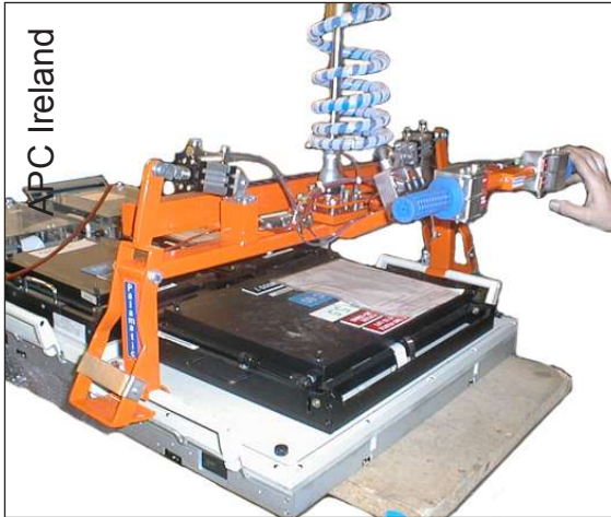
REF NO: E-PG-001 WEIGHT: 20kg FEATURES: Pneumatic power pack gripper
